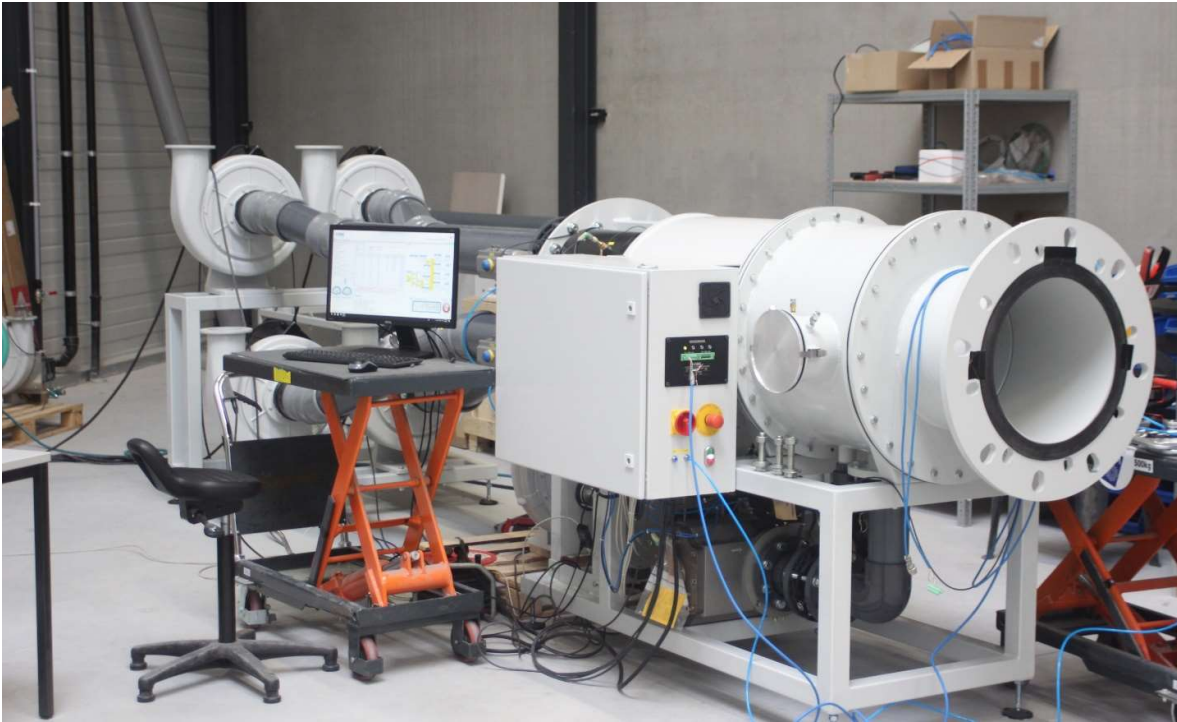
Image 2: DN150 (6") side inlet for testing rotary meters and turbine meters up to 500 m 3 /h
