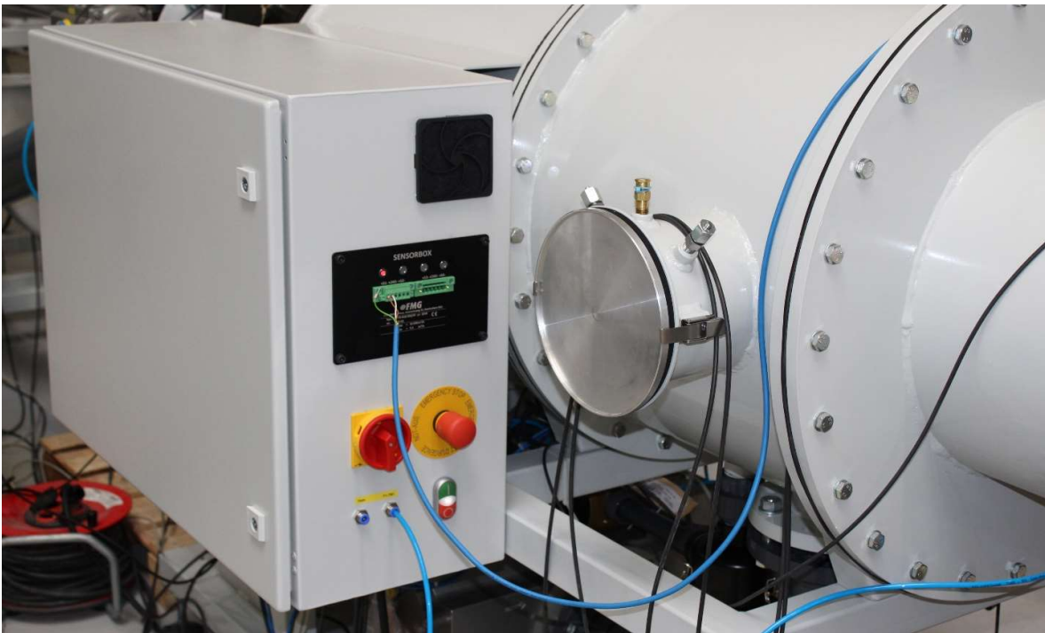
Image 2: DN150 (6") side inlet for testing rotary meters and turbine meters up to 500 m 3 /h
