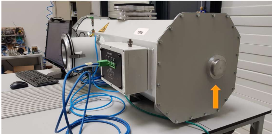
Image 4: side inlet for testing diaphragm meters
